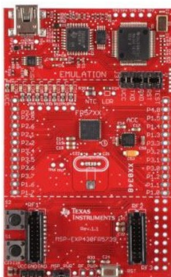
Figure 2. MSP-EXP430FR5739 Experimenter Board
