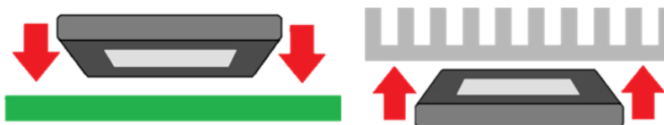
Figure 2-2. Pad-Down vs. Pad-Up Audio Amplifier
