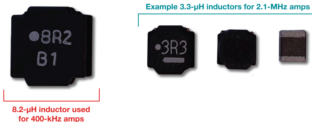
Figure 5. Comparison of inductor size vs. switching frequency.
