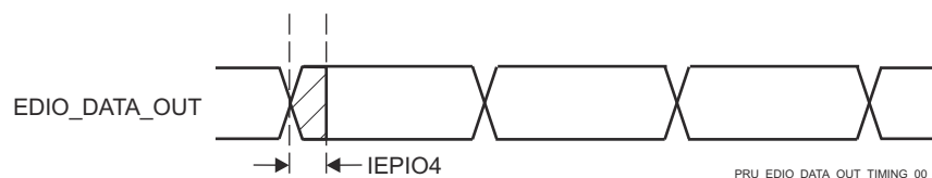
Figure 7-111. PRUSS IEP Digital IOs Timing Requirements
