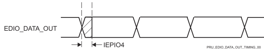
Figure 6-100. PRU_ICSSG IEP Digital IOs Timing Requirements
