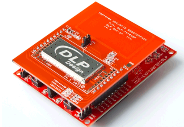
Figure 37. F5529 LaunchPad Development Kit With DLP-7970ABP NFC BoosterPack Plug-in Module
