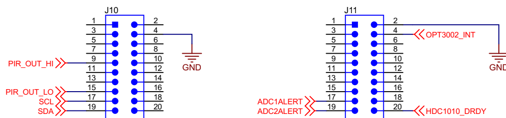
Figure 10. BoosterPack Pinout for TIDA-01069
