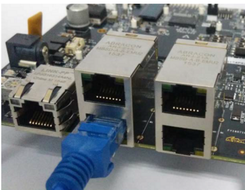
Figure 4. Connect Ethernet Cable
